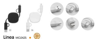
60W retractable charging cable in recycled ABS casing. Input: 2-in-1 Type-C and Type-A. Output: Type-C and micro-B (2-in-1 pin). Cable length: 80 cm. Size 5,3x5,3x1,6 cm Print technique Pad printing,DL,D01
