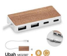
4 ports USB hub in recycled aluminium case and walnut top detail. Output: 2 x Type-A and 2 x Type-C. Input: 2-in-1 Type-C and Type-A. Cable length: 27,5 cm. Size 7,9x3,6x1,2 cm Print technique Pad printing,L,DL,DO1
